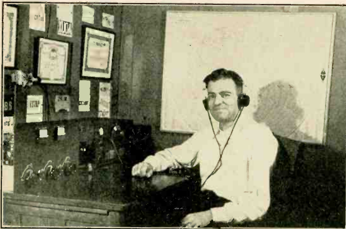
K6QYI, Doc Westervelt, Schofield Barracks, T. H. Doc used to be W3CZO and years before that he held 8UE. In this photo you will see Doc's receiver as being an HRO while the transmitter is the little 40 watt Bi-Push. However, just after this was taken Doc added a final using a pair of 35T's and now runs around 400 watts, using the Bi-Push as its driver. Most of the gang around USA claim Doc is the most consistent K6 on 20 c.w. By the time you read this QYI will be all harnessed up for 10 and 40 meters, too.
