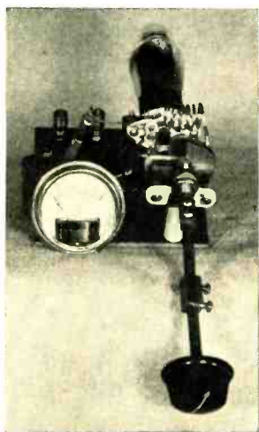
The 56-Mc. oscillator used in aligning the receiver.
