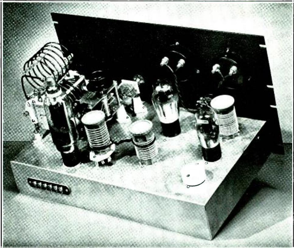
Back-Panel View of the Multi-Band Exciter, Showing Mechanical Construction
