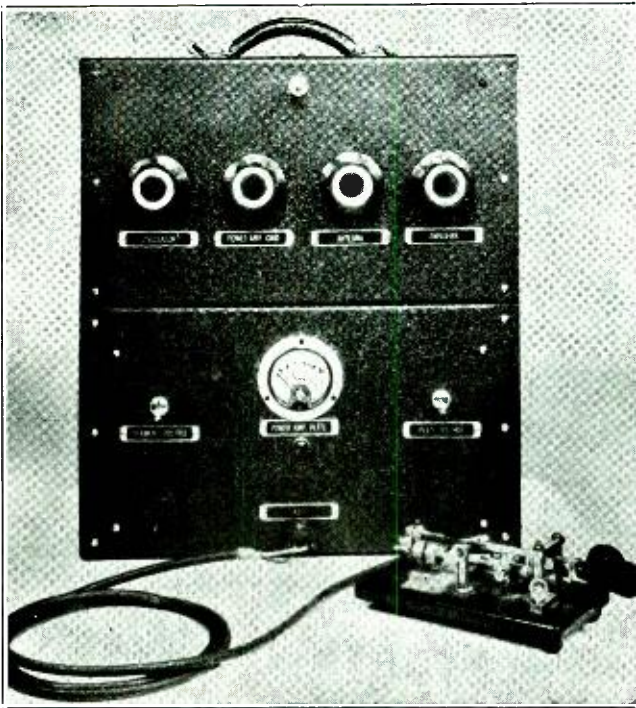
100 watts output on 3.5 mc. c.w., entirely self-contained. 39 pounds.
