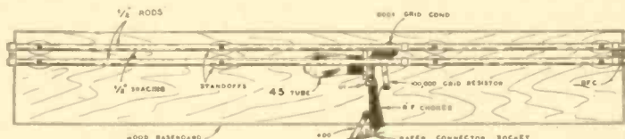
Breadboard layout of the Parallel Rod Oscillator, showing proper placement of tube, chokes, resistors and condensers.
