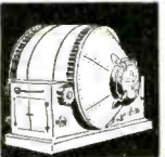
Enamels are mixed in ball mills for many hours
