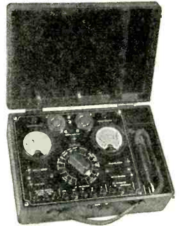
COUNTER CHECKER Type C Tests All Tubes— and makes all Voltage Tests as well.
