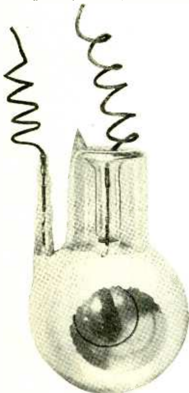
Fig. 5. Photoelectric Cell Used in Bell Laboratory Machine
