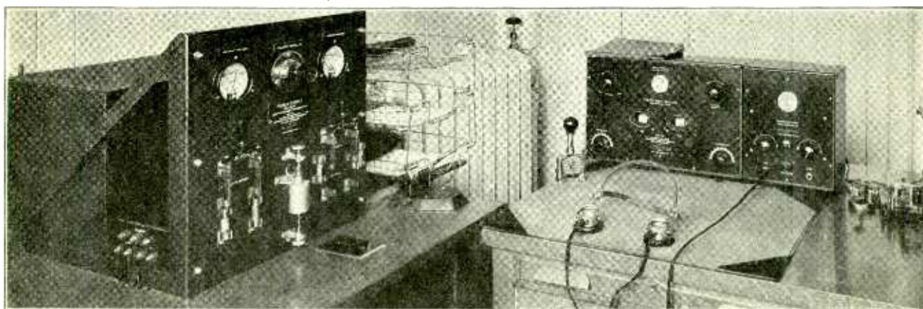
Power Panel and Receiver at KRG
