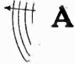
"A" is a stray field or wave, traveling toward the coil. Due to the winding all induced currents oppose each other so no current can flow. Hence no pick-up.
