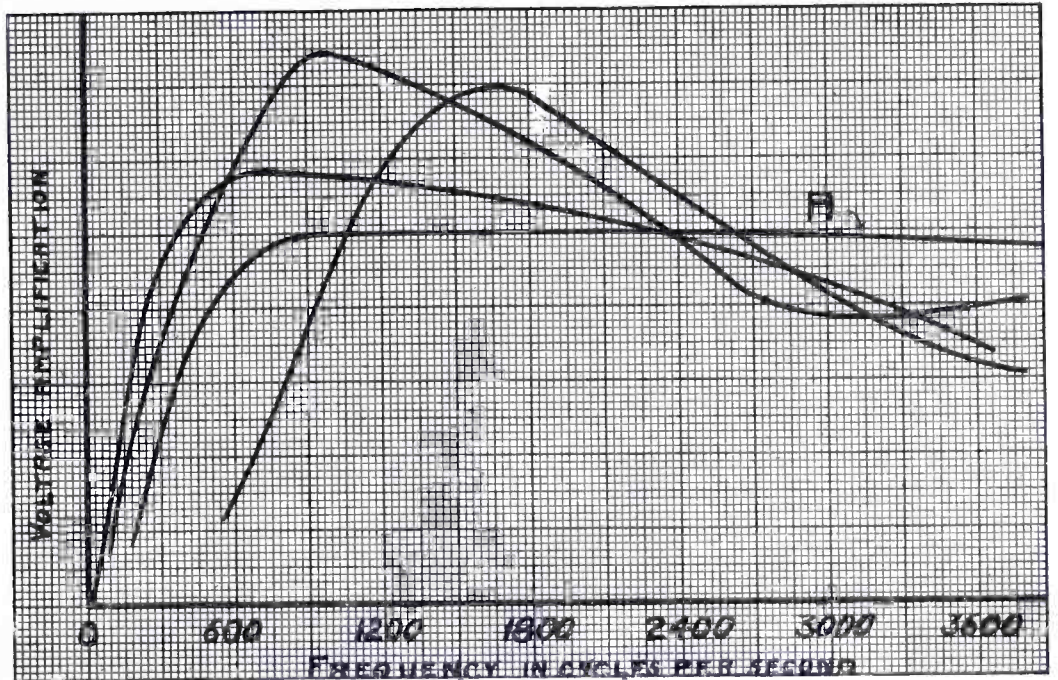
Fig. 1. Amplification Characteristics of Several Audio-Frequency Transformers, Only One of Which Is Satisfactory
