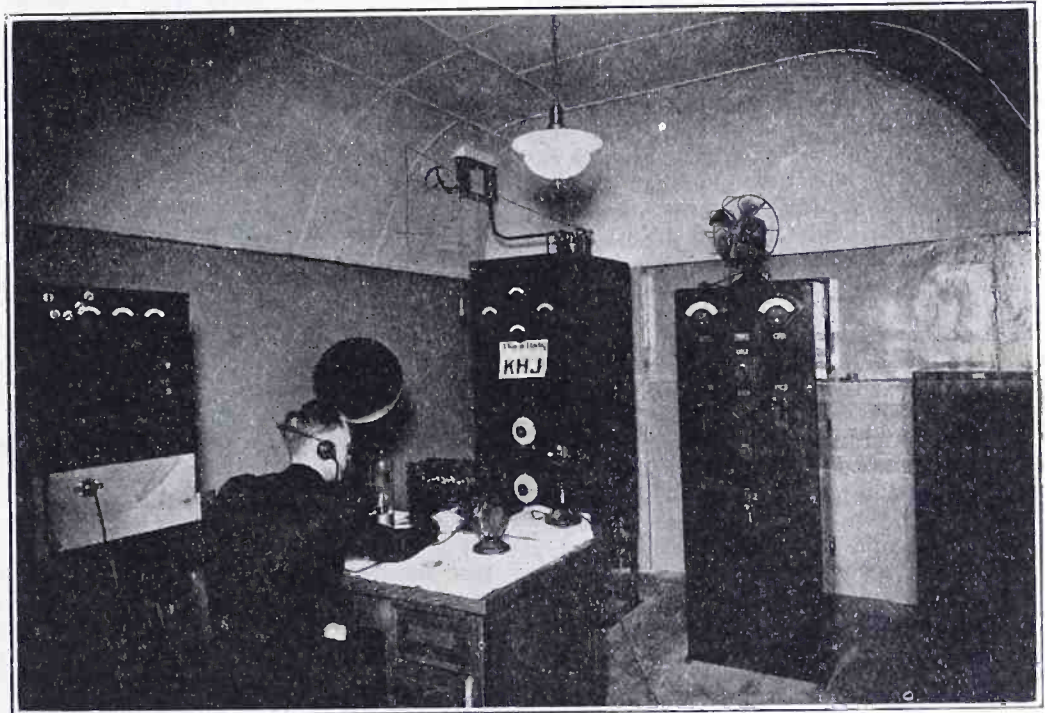
Yes, this is KHJ, . . . . . in operation. Input panel, transmitter panel and power panel, reading from left to right. KHJ, 500 watts, has done a great deal for Radio in the Southwest since November 1st. Can you see the milliammeter readings? Somewhat indistinct. However, the antenna ammeter reads eight and five-tenths amps. "Uncle John," the bedtime story telling genius, and "Cousin Bill," the humorous news reader, are on the job in the studio, a beautifully furnished room with proper broadcast accoustice. This is just the instrument room. The back in the foreground belongs to G. C. Farmer.
