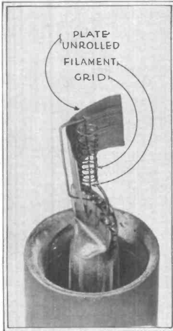
The radio vacuum tube is something like an electric light bulb. It has a filament that is lighted by a battery and two other special "elements"
