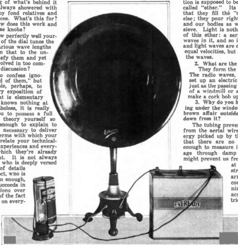
Here's a radio outfit, sketchy, but workable nevertheless. The loud speaker and "B" battery at the right form the real music and speech-making equipment. The vacuum tube and its filament battery in the center are simply the medium whereby the radio currents coming in from the left are permitted to increase or reduce the strength of the "B" battery current and thereby cause the speaker's diaphragm to give off intelligible sound waves
