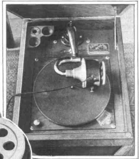
Above—A phonograph makes a good speaker, but be sure there aren't any loose parts, such as tone arm, braces or levers that can get to rattling. If they do vibrate, hold them tight with felt or cloth
