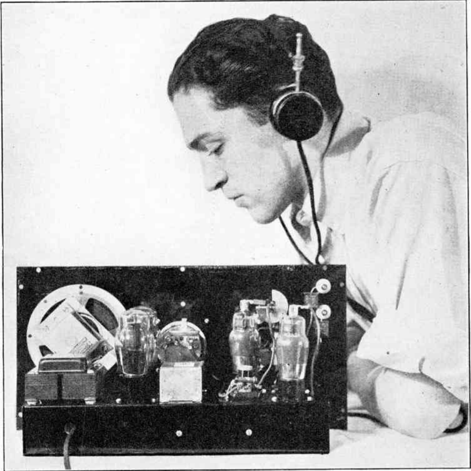
Here is the rear view of Dr. Smejkal's audio oscillator. The zero beat method of adjusting the two r-f oscillators is being used by Sidney S. Fleischman, laboratory technician. Either the zero-beat or the 60-cycle standard may be used, or both.
