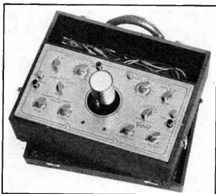
The Triplett oscilloscope.
