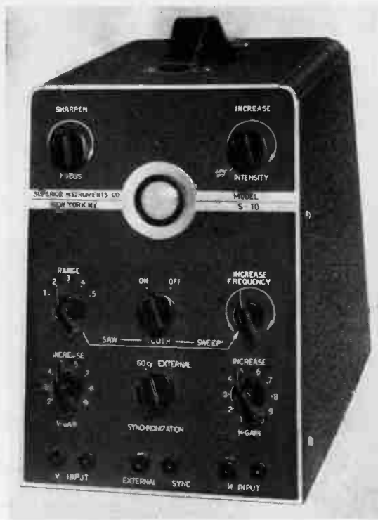
A fetching appearance marks the front view of the Superior Oscilloscope that sets the all-time record for lowest price of a complete oscilloscope with amplifiers. Cabinet is 7½" wide, 10" high, 10¾" front to back. Front panel is sloping. The 913 has an adjustable insulating hood enabling viewing in broad daylight.
