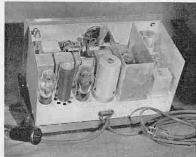
Rear view of the audiometer. All the parts are mounted on a metal chassis that fits as a unit in the outside box.
