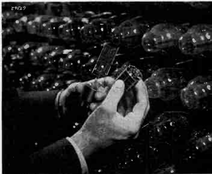
C. Depew, of Bell Laboratories, testing a tube for shock. The lines on the screen behind the swinging pendulum determine the intensity of the shock.
