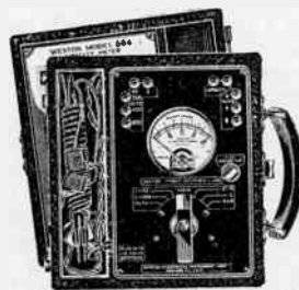
FIG. 14 Top view of the Weston capacity meter. The instrument is direct reading.
