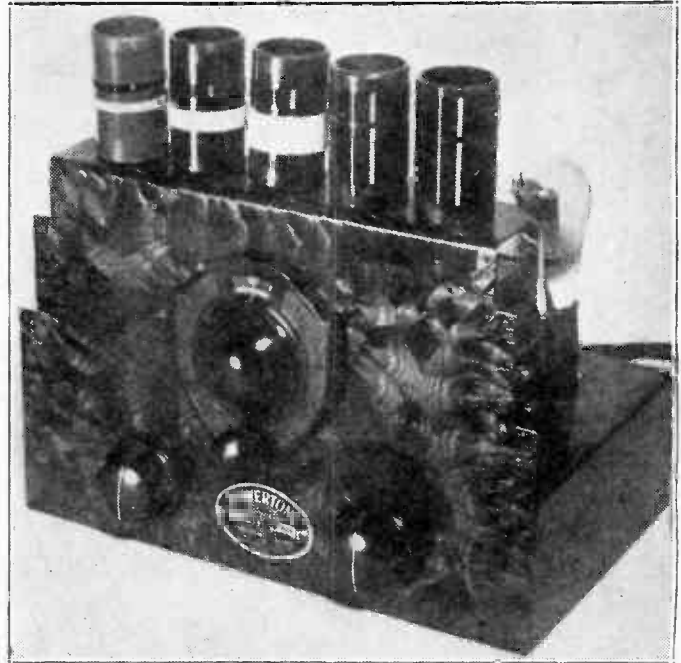
The front view of the set, showing rack for holding the plug-in coils.
