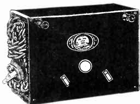
The new Bernard Universal Test Oscillator, fundamentals 135-380 kc, for lining up intermediate frequencies, 135 to 500 kc, and broadcast band, from a direct-reading dial. Special method permits calibrating short-wave frequencies. Model 30-AB, complete, with 30 tube and neon tube.....$12.00
