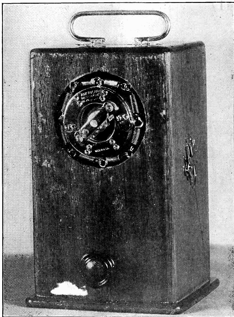
The Communicator, a four-tube portable amplifier with 2 watts output. The microphone is mounted on the front of a compact cabinet. The device may be used for office communication, store demonstrations and other purposes. See page 6.
