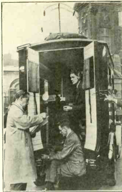
(Acme) London, Eng., radio police track down unlicensed receivers with set that picks up their squeals.
