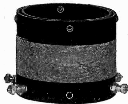
TP5 . . . . $3.00 Interstage coupler to work out of a screen grid tube, where the primary in the plate circuit is tuned, the secondary, in the next grid circuit, untuned. Tunes with .0005. Model TP3, for .00035 mfd. . . . . $3.25
