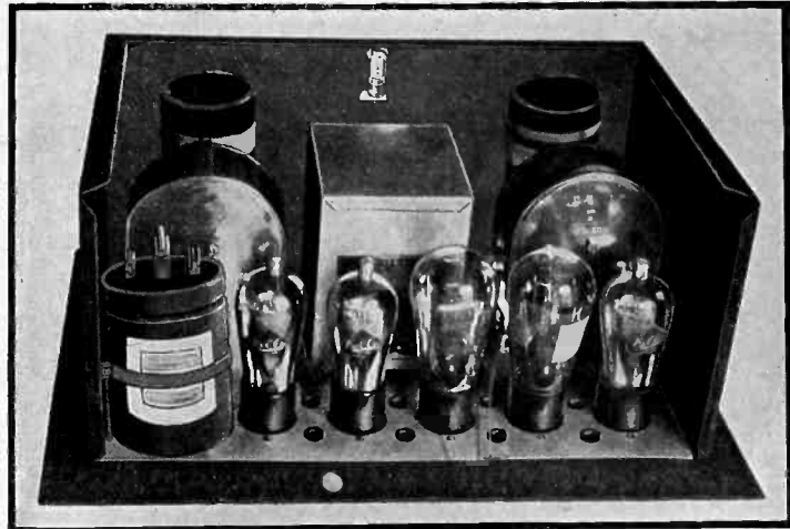
View of the HB Compact AC Model, the tubes being, left to right 224 detector, 224 first AF, 245 power tube, 280 rectifier and 224 BF. The subpanel is only 9 1/2 x 14 1/4", yet everything save the speaker is in this small space!
