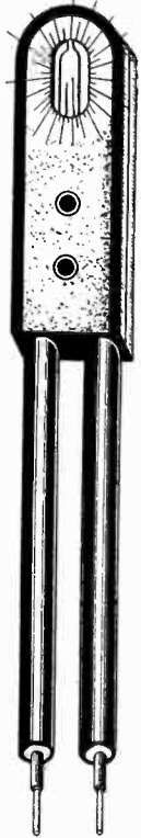
Illumination Tester, Vest Pocket Size, Shows Shorts and Opens Visually, also polarity of DC line. A Neon lamp is built in.
