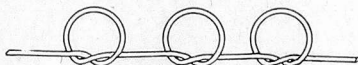
FIG. 1 THIS SHOWS THE PROPER WAY OF SEWING A CABLE. EVERY INCH OR SO A KNOT IS THROWN AROUND THE BUNDLE OF WIRES.
