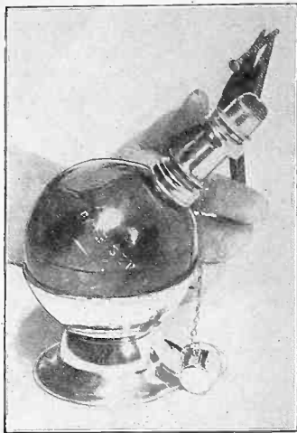
A METAL SCREW HEAD ON THE PANEL WILL BE MUCH MORE ATTRACTIVE IF IT IS BLUED. HOLD THE HEAD IN THE FLAME OF AN ALCOHOL - BURNING JEWELER'S LAMP, AS IS DONE HERE, UNTIL THE HEAD IS BLUE
