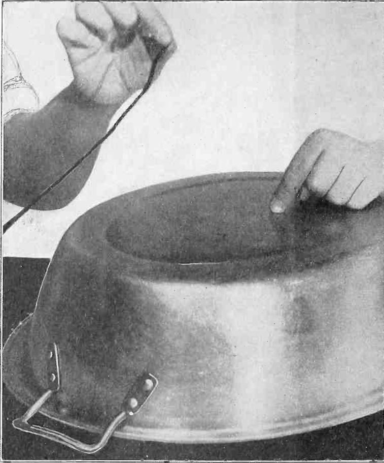
A METAL DISH PAN CAN BE MADE TO TALK BY CONNECTING THE POSITIVE TERMINALS OF THE B BATTERY TO IT AND THEN GRASPING THE LEAD FROM THE POWER TUBE PLATE IN ONE HAND AND TOUCHING THE DISH PAN WITH THE OTHER. IF THE HANDS ARE MOIST A SHOCK MIGHT BE EXPERIENCED
