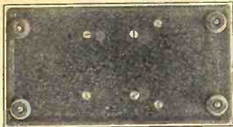
FIG. 4, the bottom plate. The screws holding the rubber feet, hold the transformer (left) and the condenser bank (right).
