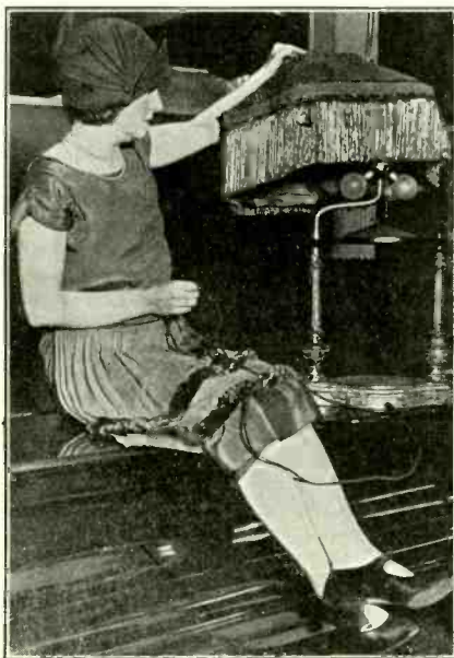
A NEW lamp loud speaker which uses a paper cone instead of a horn. Miss Nancy Slavin of Brooklyn, is demonstrating what it looks like when the shade is removed. (Kadel & Herbert.)
