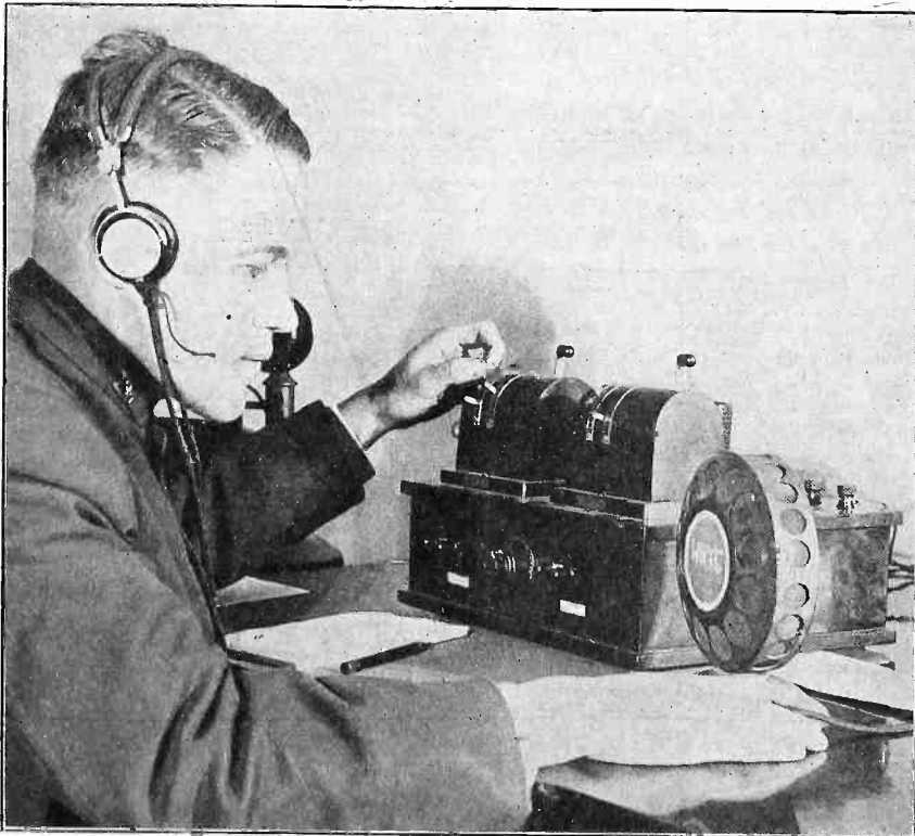
A DEMONSTRATION at Police Headquarters, New York City, connected by land line to station WNYC. The radio signalling device is shown in transmission work. When the key of the signalling device is closed a signal is flashed to all of the police stations and traffic booths throughout the city, which are equipped with receiving sets that are then tuned to WNYC's wave. This rapid means of communication is intended to help the police in watching and capturing automobile bandits. (International Newsreel)
