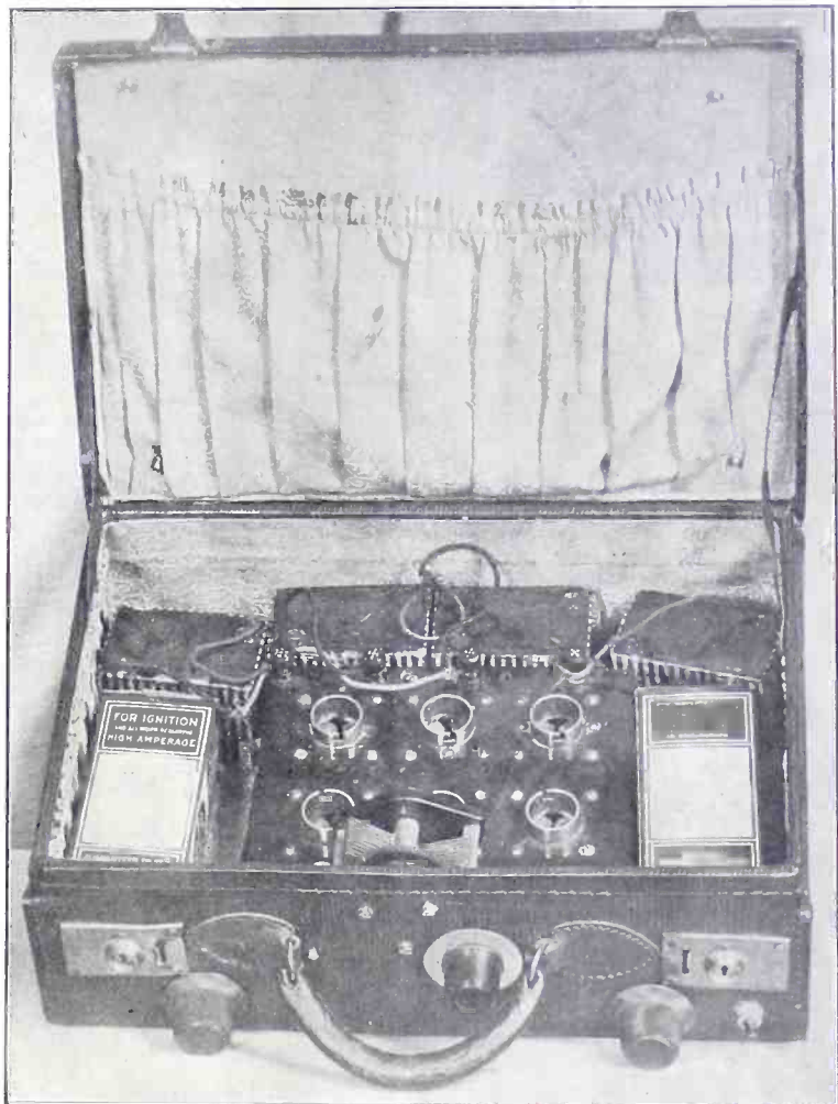
FIG. 2, the set in the carrying case, with the contents exposed. The variable condenser is at left of the dial because only the vernier device is used, there being no direct actuation of the main shaft. The standard system would do just as well, however. The midget B batteries are shown in the rear. Wound under the lining of the cover is the loop.
