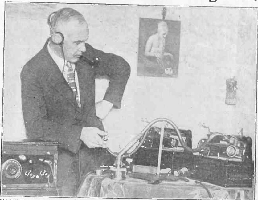
“CANNING” RECEPTION —N. J. Wilcox, of San Francisco, has perfected an ingenious device for recording a radio program. The set is hooked to the dictaphone, without any intermediate device. Mr. Wilcox says the greatest difficulty was in harmonizing the dictaphone with the radio voice vibrations. He is the only person in the country known to have overcome the problem. The President's pre-election speech, on two cylinders, was presented by Mr. Wilcox to the Chief Executive.—(Wide World)
