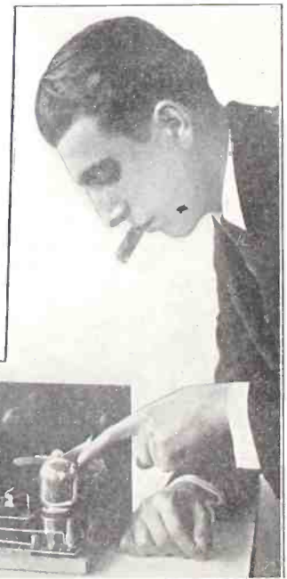
THE AUTHOR "points with pride" to the power tube in the last stage, a Daven Mu-6. The two tubes to the left thereof are hi-mu (20-mu), while -01A tubes are used for the two RF and detector stages. The Lemnis Coils are in the moulded Bakelite containers of peering-glass shape. (Fig. 4).
