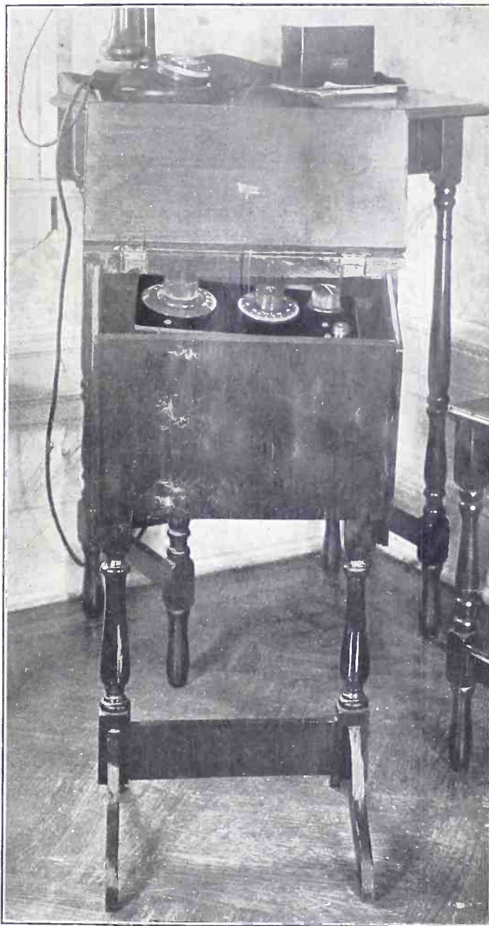
THE MIDGET SET installed in a sewing cabinet, Priscilla model. The view shows the completed set as it looks in the home. Two lids, one for front, one for back, facilitate operation of the set and attention to the batteries. The whole outfit is self-contained. The cabinet is of handsome appearance and looks very attractive even amid exquisite parlor furniture. (Hayden.)
