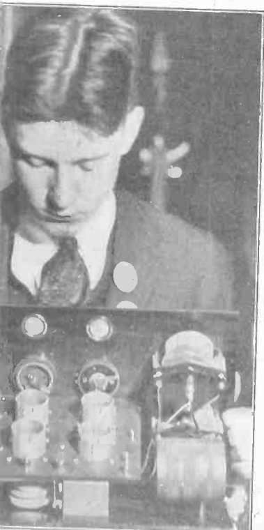
emblem a Super-Heterodyne, with the eight and the transformers beneath.
