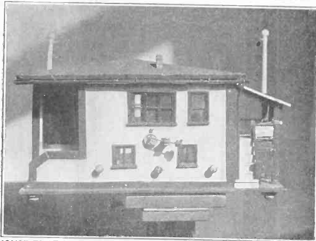
HOUSE THAT JACK BUILT is really an RF set, using crystal detector. It looks like a house and works like a charm. The constructor was John Neis, of 1533 Wolfram Street, Chicago. (Foto Topics.)
