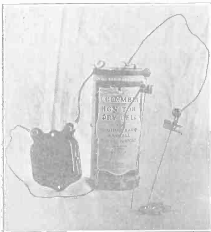
TESTING DEVICE —Even the humble hatpin may be used in testing for short or open circuits. In photo the positive A is connected to a clip on the pin, the negative A going to one side of the buzzer, the other side of the buzzer to another pin. The beaded tips are good insulators. A fixed condenser is in foreground, prior to a short-circuit test.
