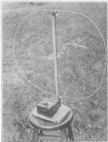
(Miller News) THE CROSSED COIL radio beacon guides the ferry boats across San Francisco Bay in foggy weather. The beacon consists of two coil antennae across each other at an angle of 135 degrees.
