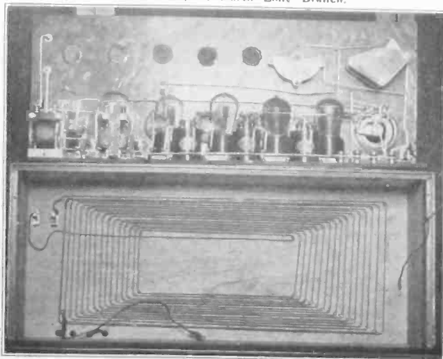
(Kadel & Herbert) REAR VIEW of a remarkably efficient receiver designed and constructed by Rutledge Mayo, of New York City. Using three stages of radio-frequency, detector, and two stages of audio-frequency amplification, Mr. Mayo has picked up stations 1,500 miles distant on the loop. A double circuit jack mounted on the panel enables the use of an outdoor antenna and ground simply by plugging in.
