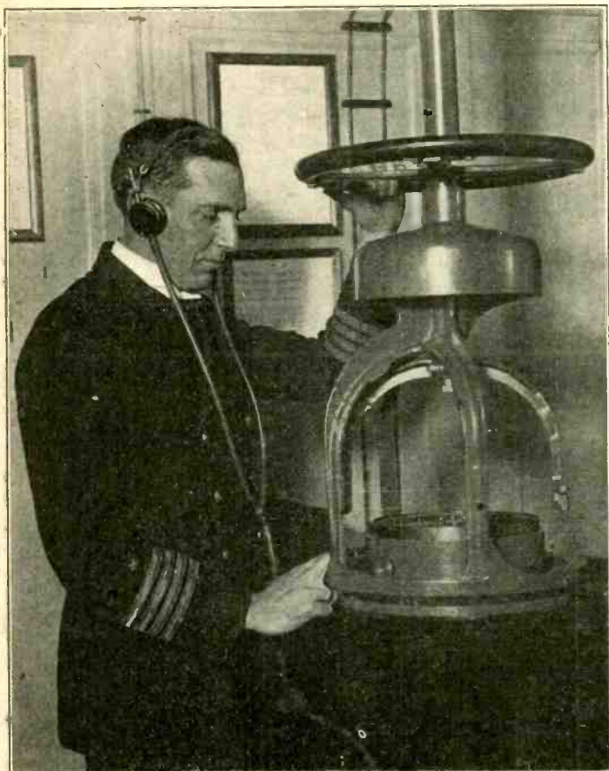
(C. International) Staff Commander H. C. Fish, of the S.S. "Leviathan," operating the ocean greyhound's radio compass which has proved of great aid in finding the ship's location when a fog closes in. Due to the use of radio-frequency and special tuning circuits used for this work, the compass is accurate to a remarkable degree, and when the percentage of error is known, settings may be taken almost as accurately as with the compass and sextant.
