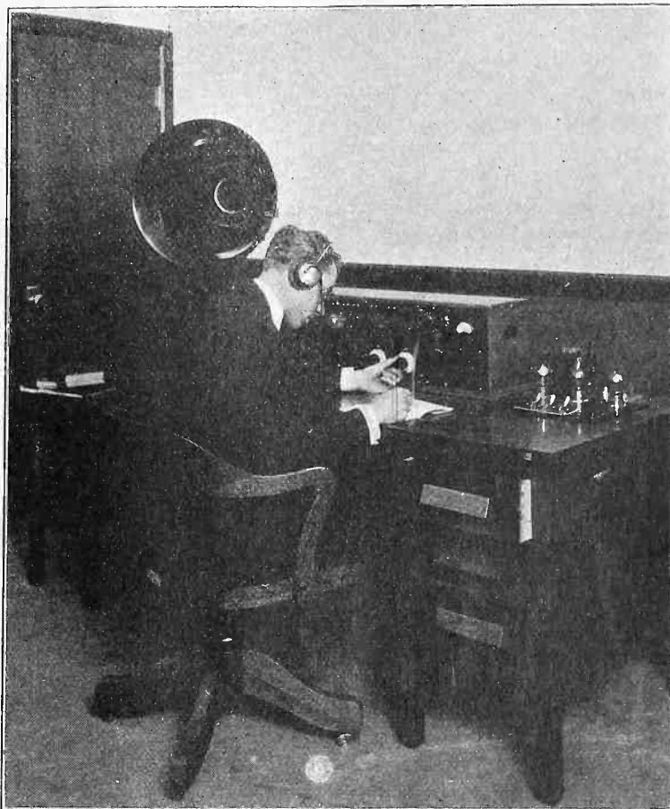
Radio sending and receiving set designed and built for the Piedmont High School. The apparatus is installed in an ordinary office desk.
