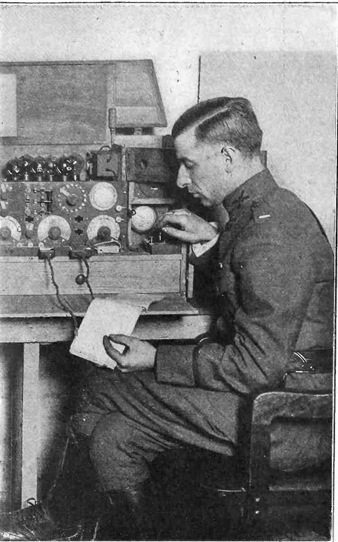
Testing out the famous "Porte E10" French Army portable messages to planes manoeuvring over the field to litter. Note the apparatus on the left, showing the complete receiver and transmitter, capable of being driven generator. Each machine has six tubes, and a triple pole double switch seen directly under the bank simplifying matters considerably. Note also the jacks, to be inserted in the right manner, due to the slots cut a certain it a wonderfully compact but at the same time marvellous.
