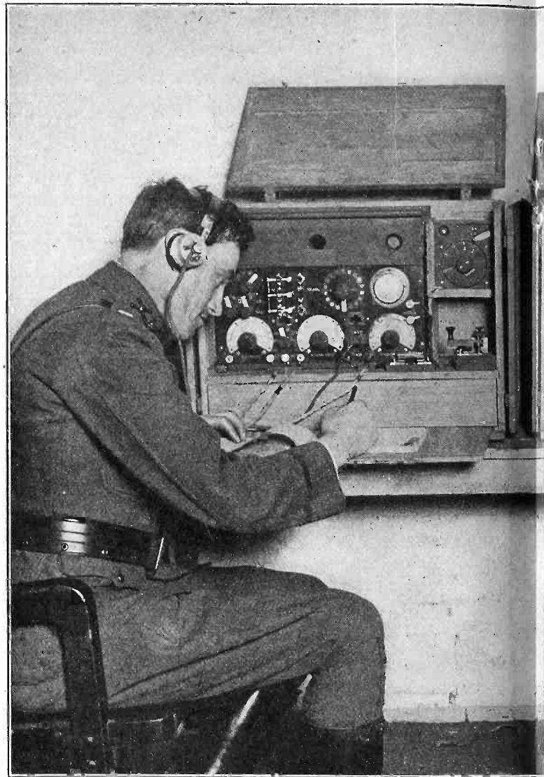
(C. Kadel and Herbert) The 212th Anti-Aircraft Artillery, Radio Division of the Signal Corps, is testing a portable radio receiver and transmitter. They are transmitting and receiving to ascertain the efficiency of the French short wave receiver and transmitter. The portable wave meter in the upper right hand corner. Each machine is easily carried in a scout plane, and operated by means of a wave change-over from transmitting to receiving is made by means of a change-over of tubes. The same tubes are used for reception and transmission which are of such construction that a phone or microphone can be used in either way. The apparatus can also be used for telephone work, and is extremely flexibly.
