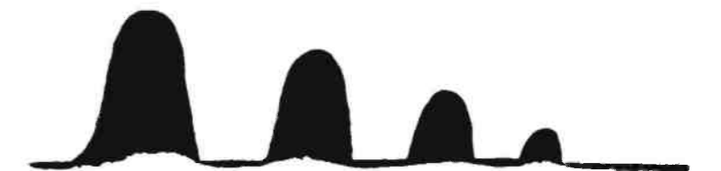
Figure 2. After passing through detector, wave of Figure 1 has been reduced to this form. The negative wave has been strained out by the crystal.
