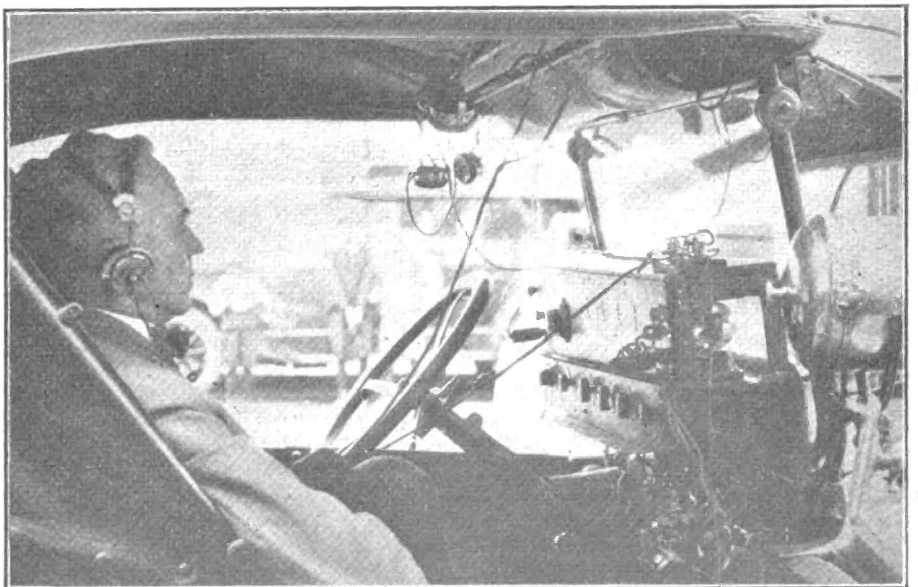
An automobile with a loop aerial in front of the wind screen and a receiving set on the dashboard recently made its appearance in the streets of New York. Crowds gathered wherever it stopped and listened to the music of broadcasting stations. Mr. and Mrs. J. C. Davenport, owners of the car, were testing out their new radio set, known as the "Dashboard Special." They had just completed a forty-thousand mile tour and were about to leave on a second tour of indefinite duration. The upper picture shows the "Dashboard Special" in front of the Pennsylvania Station, New York City. The lower picture shows Mr. Davenport and the arrangement of his car's fine radio equipment.
