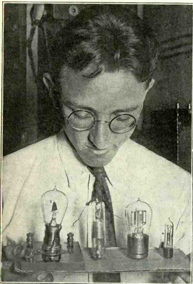
(Both photos: C Kadel & Herbert News Service) Four stages in the evolution of the vacuum tube. From left: Fleming valve; De Forest tube; Radiotron; Peanut tube.
