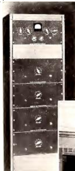
Amplifier panel of this 56 speaker installation.
