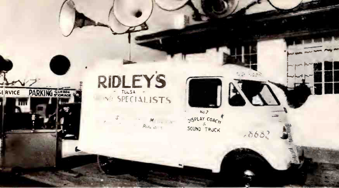
Latest addition to the truck fleet of the sound specialist, R. P. Ridley, of Ridley's, Inc., Tulsa, Okla. The truck mounts six 6-foot trumpets, has a 100-watt Class A amplifier.
