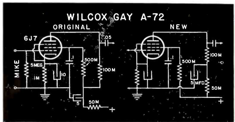
Circuit diagram changes shown at right prevent oscillation at high volume levels.
