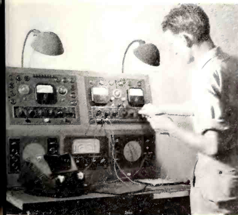
↓ Auto radio sets are quickly and systematically handled with equipment having necessary power and speaker plugs. Test bench may also be rolled to side of car.
