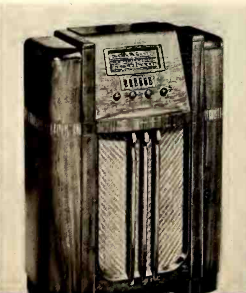
Stewart-Warner model 01-6A7, 3-band, super, lineardial, line antenna, push-button.
