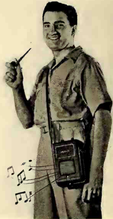
Motorola's "Sporter"—compact camera-case portable. Weighs under 5 lb. Shoulder-strap forms loop antenna.
