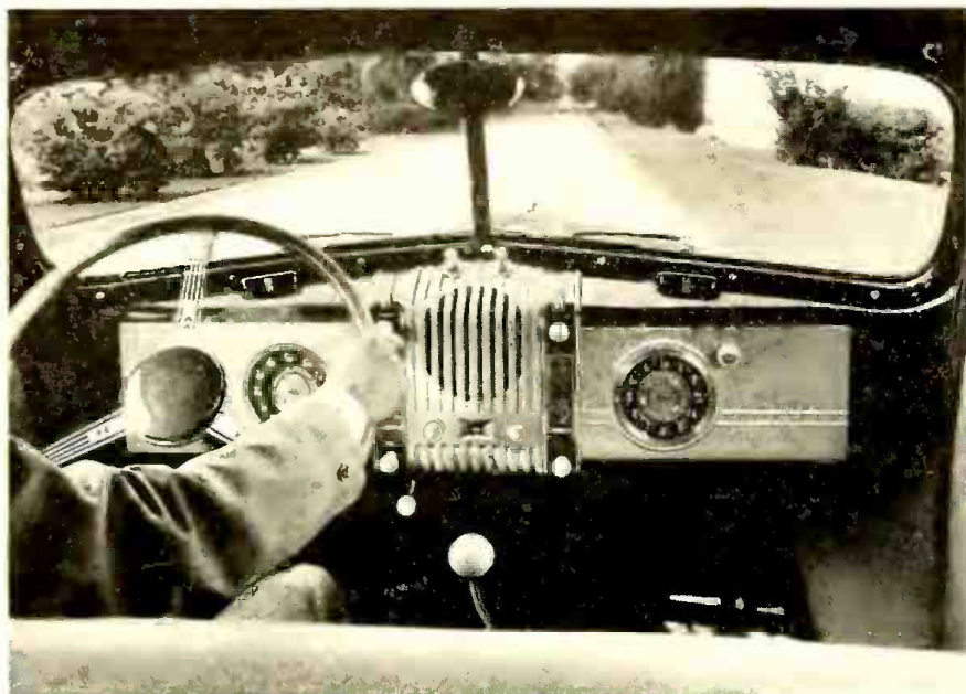
Auto-radio controls now become an integral part of the dash design, yet are available for nearly all cars in models sold by radio trade.
