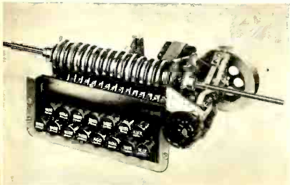
The insides of Stewart-Warner's tuner are mechanical in operation rather than electrical. The stations are set from the front of the dial.
