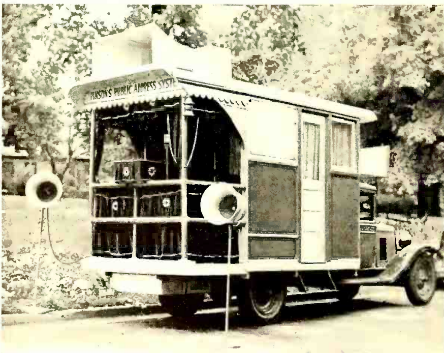
Fancier than the usual truck, this one by H. M. Pinson, Lexington, Ky., has special platform lights, sleeping quarters, and p.a. gadgets to attract politicians, evangelists, advertisers, lecturers, singers, etc.
