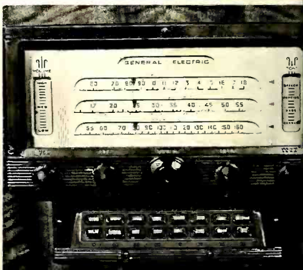
General Electric's push-button system turns on the set as well as tunes in the station.
