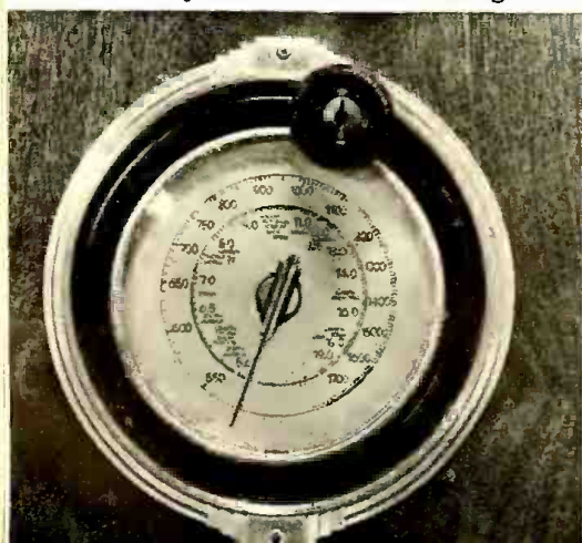
Below is Philco's dial used with the concentric system of automatic tuning.
