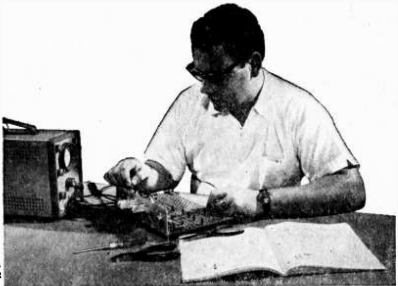
Performing transistor experiments on programmed breadboard—using oscilloscope
