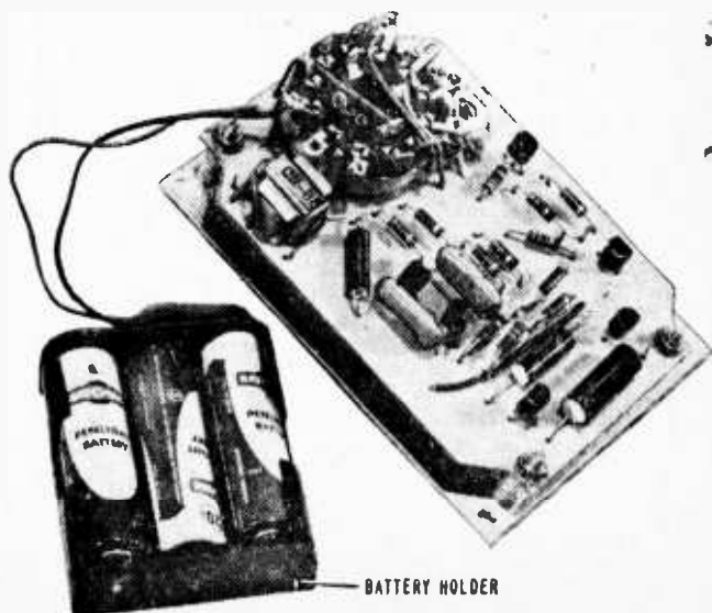
The printed circuit board mounts on spacers behind the case's panel. All wiring (top) is completed before final assembly. (See below.)
