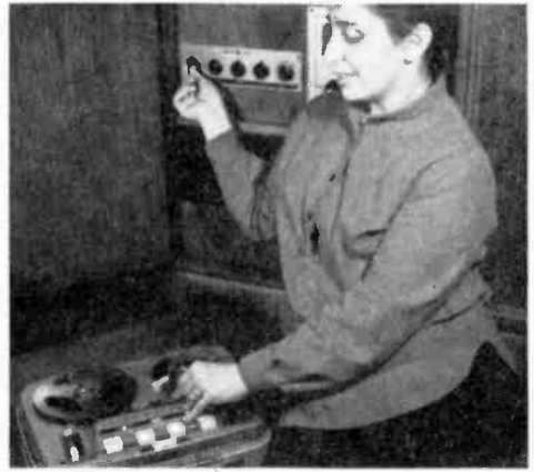
12 You can by-pass tape recorder's preamplifier and clip-lead connect directly to the phono input of your amplifier to check out tape preamp.
