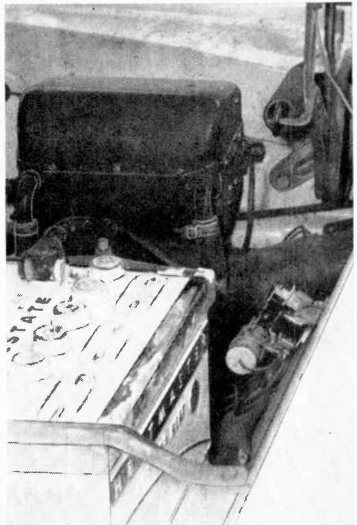
FIG. 9: Mount the transmitter relay under the hood.
