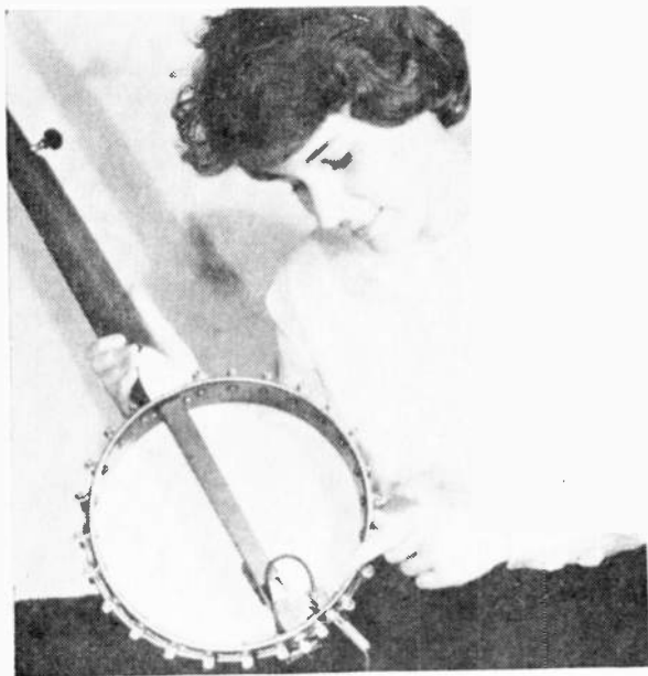
Fig. 1: Rubber-covered pickup is mounted on underside of head, beneath bridge. Cardboard shims hold in place.
