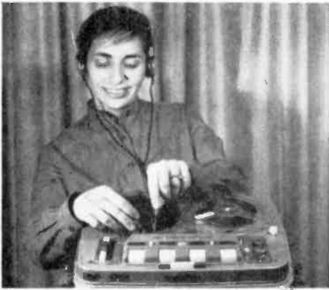
11 If unit fails to record, bridge terminals of record head with a pair of earphones to isolate the trouble. You should hear the program material.
