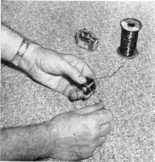
FIG. 5: The coil of the transmitter relay must be completely stripped and rewound with No. 18 Formvar.
