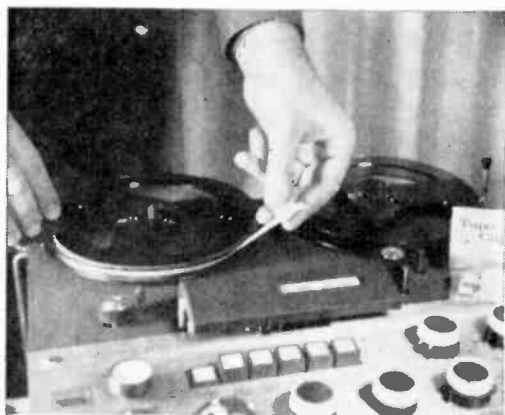
Fig. 6: Using 3-M tape clips will keep the tape end on the reel where it belongs. Keep tape from spilling during storage or transit. Removes easily to use.
