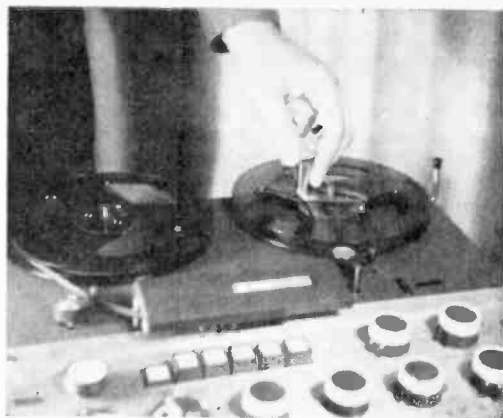
Fig. 4: Threading tape onto take-up reel is always a problem for neophytes. Robins' crank-type threader solves the problem for the "all-thumbs" tyro.
