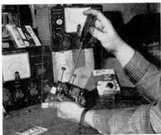
FIG. 7: Reassemble frame, replace screws "A" and "B."
