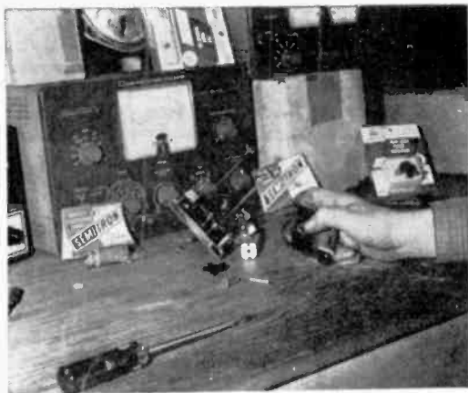
FIG. 5: Using thumb and gentle pressure, push out the rotor assembly. Do not hammer; push it carefully.
