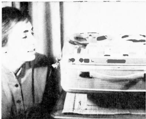
Fig. 13: Check for reel-warpage at eye level while reel turns. Any warp will quickly become obvious, reel eliminated before it could damage tape.
