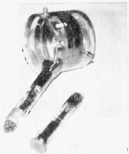
Fig. 2: The large iconoscope was used as a camera tube in surplus drone planes. Smaller vidicon does same job.
