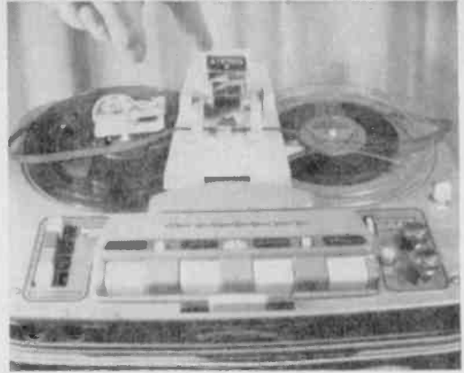
Fig. 9: Robins splicer has two locking levers that hold tape firmly in place during editing and splicing operations. When tape ends are in position . . .
