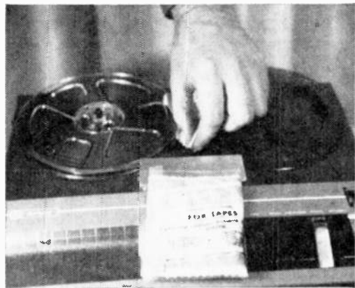
Fig. 14: Silicone jockey cloth can restore freshness to older, dried-out acetate base tapes. Simply make a loose fold over tape as it travels in machine.
