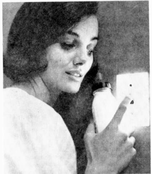
Fig. 2. Wall switch glows for over five years for under five cents per year. Lights when switch is off.
