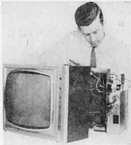
Fig. 9: Servicing is simply a matter of removing back, sliding chassis toward rear for accessibility.
