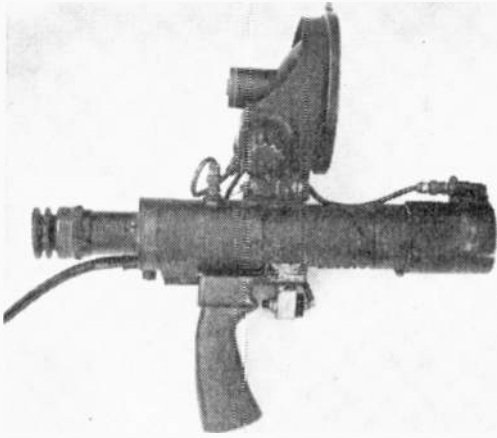
FIG. 3: Famed sniper scope is now an excellent police weapon with its built-in, infrared searchlight. A well adjusted scope can "see" up to 300 ft., but it still isn't up to the Army's new night vision equipment.
