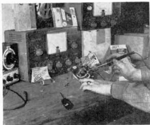
FIG. 8: Reconnect the wire leads to the motor coil soldering terminals and replace the unit into the radio.
