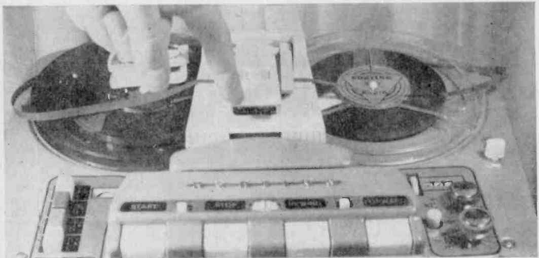
Fig. 10: Cut! The splicer cuts a 45° diagonal, in both pieces of tape. Apply the splicing tape over the cut, move the cutter head to trim, and press again. Result is "waist" cut, hence name "Gibson Girl."
