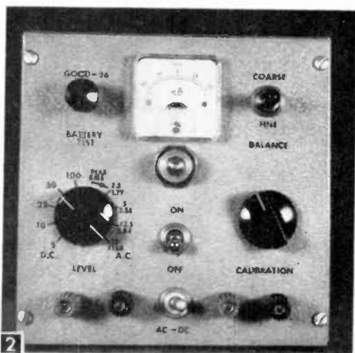
Notice on the front panel the peak and rms dual calibrations of the ac voltages.
