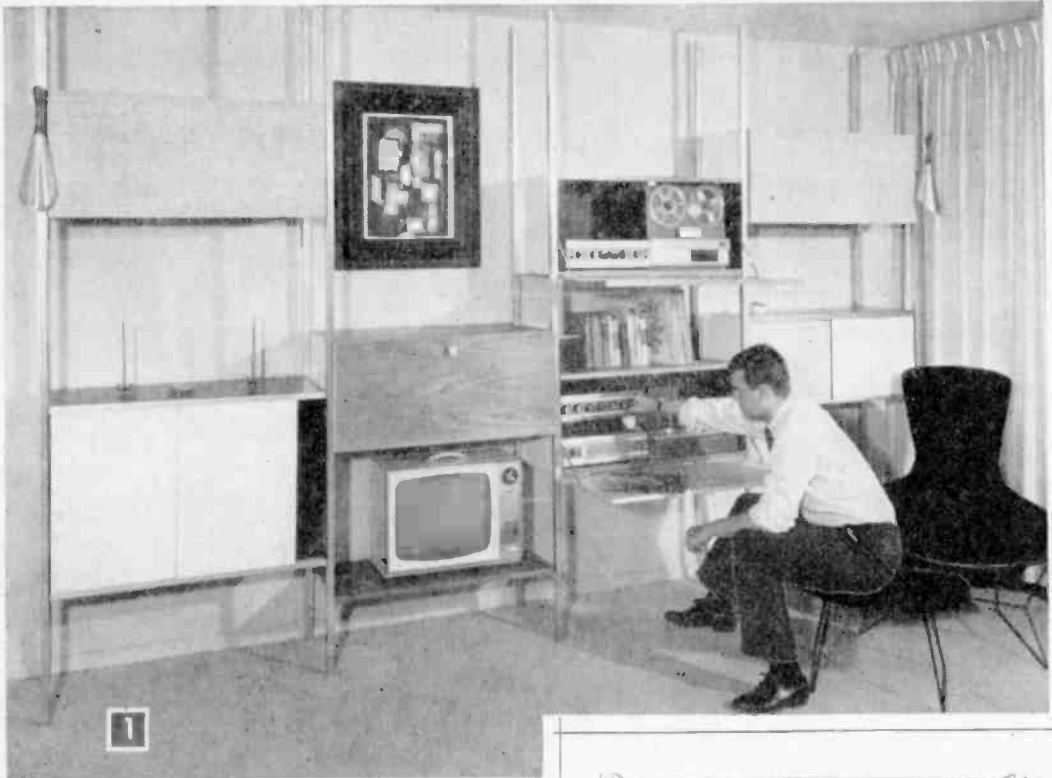
Stereo speakers are mounted in the two baffles at the top left and right. Installation has extra space for future additions, is easy to move, and does not mar walls, ceiling or rug. Room divider (A) is alternate design.
