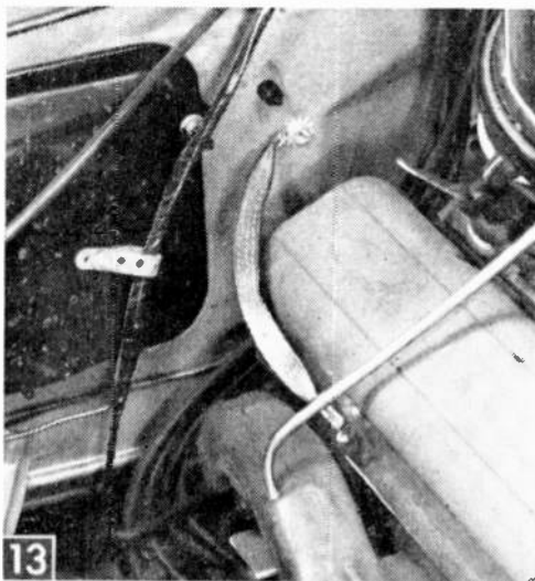
Metallic straps are available in various lengths for grounding parts in the engine compartment.
