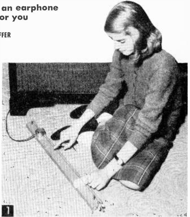
1 Connect the one string electric guitar to the phono plug of your amplifier, radio, TV set, or tape recorder. Be sure that your set is properly grounded for safety.
