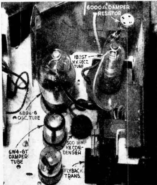
Photo C. Close-up of H.V. section. If set needs new H.V. "flyback" transformer, disconnect one wire from damper resistor. Replace original 500 mmfd condenser with new unit rated 15,000 volts. Many sets need only a trimmer attached to H.V. transformer as shown in Fig. 5.
