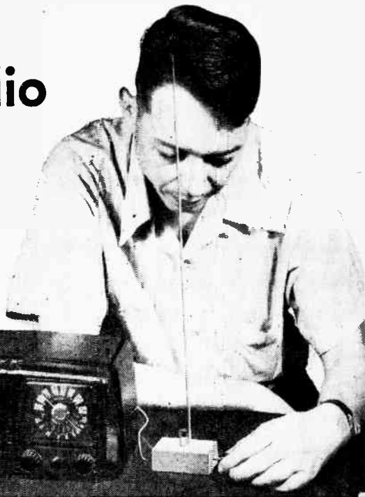
Fig. 1. Long-distance stations come in with amazing power with DX Tuner. Whip-antenna is a piece of coathanger wire about 16 in. long.
