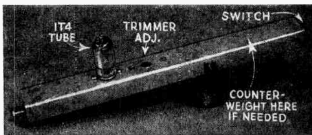
The tube may be pulled out when pickup is idle. Note that arm merely rests in forked swivel base. For LP records, add a counterweight to arm if needle pressure is excessive.
