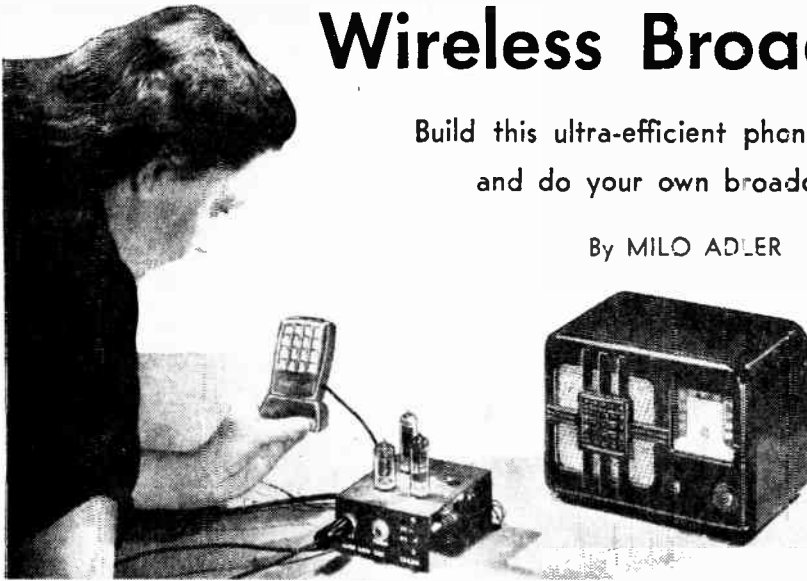
Fig. 1. Wireless broadcaster connected to mike. Radio in background will receive broadcasts from this phono oscillator from as far away as 50 ft.
