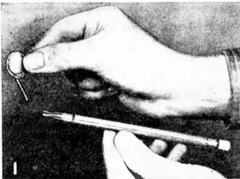
Fig. 1. Clamp a small dental mirror in the pencil, and use it to identify hidden radio parts' values or examine nameplates on appliances.
