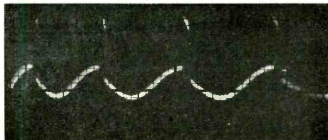
Fig. 5A—Oscilloscope photo of wave form at the plate of the horizontal mutivibrator. (Fig. 4)
