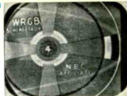
Fig. 2—Horizontal fold-over usually caused by too long a horizontal retrace time. Courtesy G.E.
