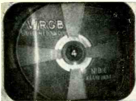
Fig. 1—The faint white line at the left may be due to a defect in the damping circuit. Courtesy G.E.
